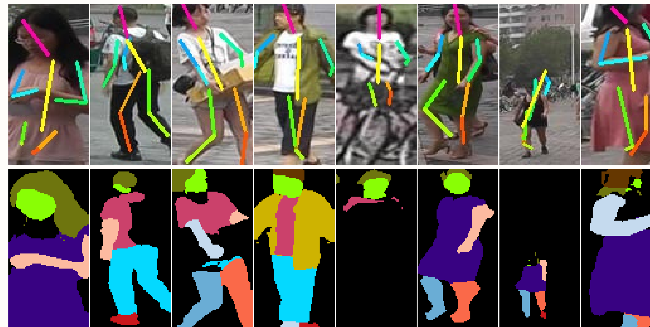
Automatic annotations on the Market-1501 dataset for pose estimation (top) and part segmentation (bottom).
