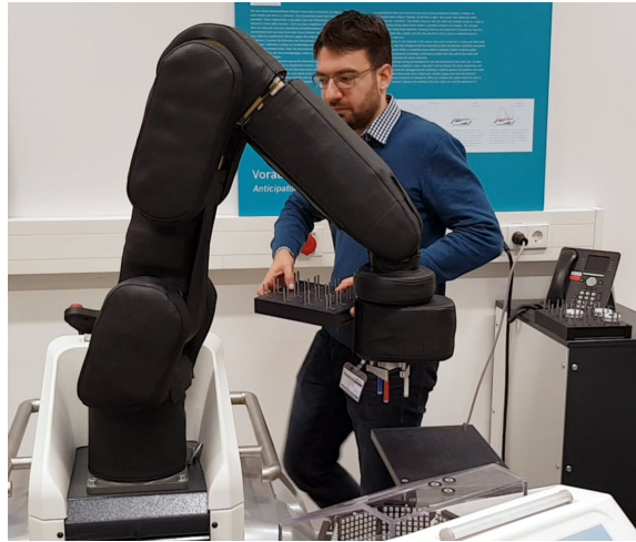
Figure 4.1: Example of partial occlusions in the context of shared human–robot workspaces. Note how easily we humans can guess the rough pose of the person behind the occlusion. Can current 3D human pose estimation methods do that as well?
